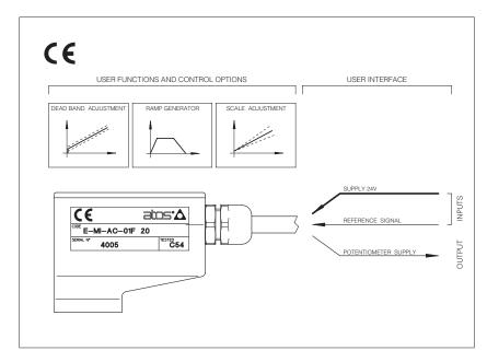
1 MODEL CODE 01F E-MI AC set code E-MI = electronic driver plug format as per DIN 43650 Series number AC = for proportional valve without transducer Options: standard symmetrical ramps /RR = adjustable dissimmetrical ramps, adjustable dither, suitable also for current signal 0÷20 mA = pre arranged for double solenoid valves 01F = for single solenoid proportional valve
